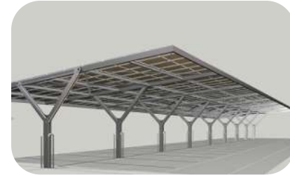
Photovoltaic parking covers
